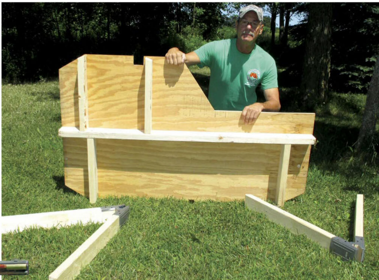
The tabletop is constructed from \frac{3}{4} -inch plywood and 2x4 supports. The removable 2x4 legs are made using metal sawhorse brackets.
